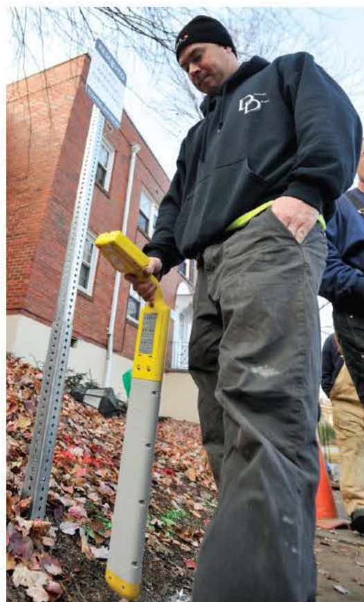
Wes Fogelman uses a drain line locator from Rycom Instruments to find a sewer line.
